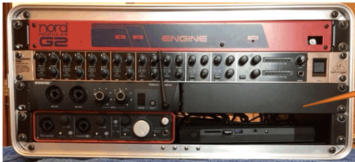
Gig Rack, including Cantabile PC, audio interface, IEM transmitter, Mixer, Nord G2 Modular rack (With DMXIS, USB hub and MIDI hub not visible)
