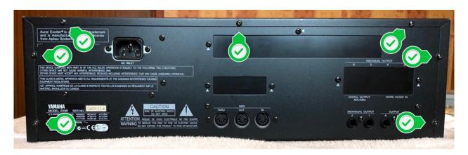
Now you can remove the case, and you will have the following view. The front of the EX5R is towards the bottom of the picture.
