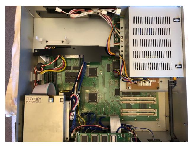
The battery is right under the floppy drive, which will need to be removed.
