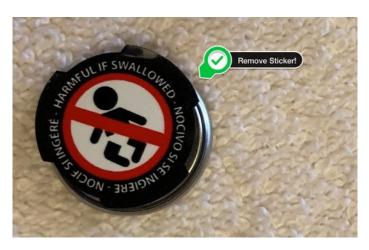
The battery holder in my EX5R is spring loaded. To remove the battery, you need to gently push the battery towards the back of the of the EX5, and gently tilt it up as well as you do so, A small screwdriver is ideal for the task, and you can just about make mine out at the front of the shot, and where I was gently levering. You can see the spring at the top of the battery holder that you need to compress.
