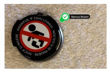
The battery holder in my FS1r is spring loaded. To remove the battery, you need to gently push the battery towards the back of the of the holder (so push leftwards in the picture above), and gently tilt it up as well as you do so.
