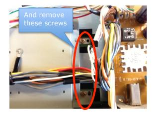
You'll need to slide and angle the housing to remove it. I also found that in my synth, the rear of the housing was catching on the screening foil underneath it, so it wouldn't move out easily until I had freed it.
