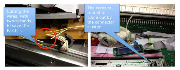
As mentioned, earlier, this 5V supply is outside the quoted range of the new Display's LED backlight, so we need to simply drop some voltage. This is done by putting a resistor in series with the negative line of the supply. Again, I elected to use a 1K trimmer rather than experimenting to find the right value.
