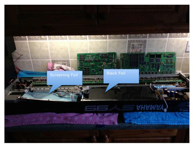
Removing the boards reveals screening material, which also needs to be removed. The black plastic under the DM2 board is easily removed, just note how it slots in the frame at the front of the keyboard.
