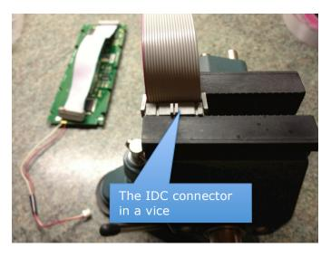
Note that you need to get the orientation of the plugs on the cable correct, to match the connector keys either end. Use the existing display (in the foreground in the picture below) to get this right.
