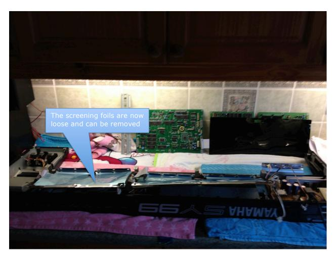
With the keyboard removed, the screening can now be removed, which will reveal the next layer!
