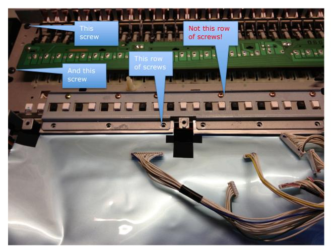
There are also some small screws on the screening by the PSU that need to be removed.
