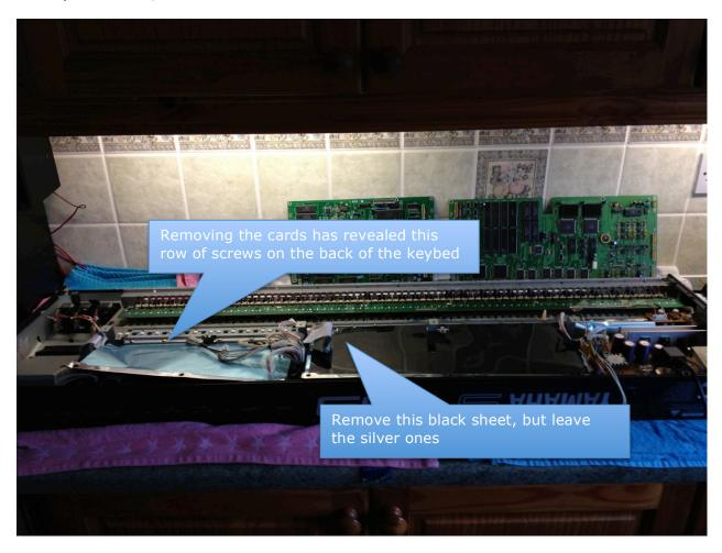
This is as far as you need to go in terms of removing circuit boards for this repair.
