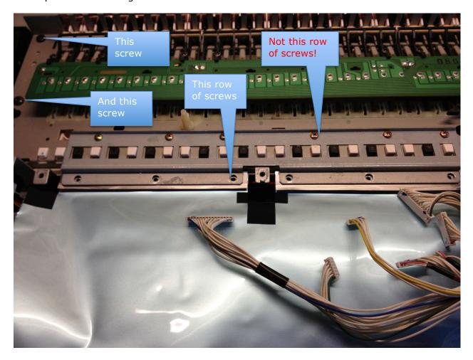
There are also some small screws on the screening by the PSU that need to be removed.
