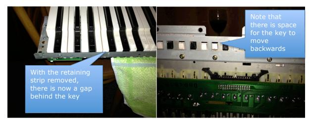
So, to remove a key, you now simply push it backwards and it will spring upwards on its own. If you are removing a black key, you will need to remove the white keys either side of it as well.
