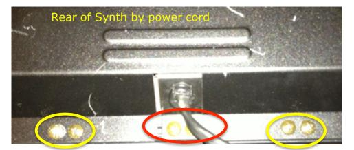
Once all of the screws are removed from the rear cover gently prise the cover away from the synth, lifting towards the front of the synth.
