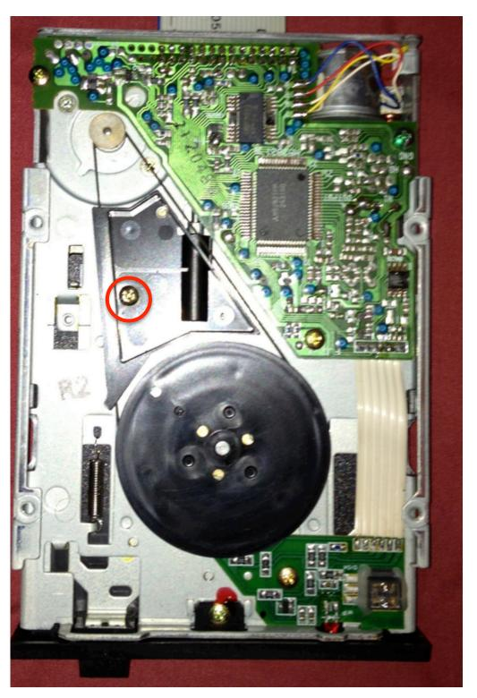
Once this screw is removed, the belt guard lifts off, and you can now remove the old belt and fit the new one. When fitting the new belt, take care not to stretch it too much, and ensure it is not twisted.
